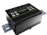
MDRX-AURA-XX X = 02, 08, 32 (ports) MADRIX Luna 2, 8, 32 port universe Artnet to DMX interface. Programmable for playback and live support (Online or Offline option)
