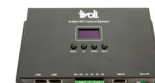
ARTNET-S-X-SPI X = 4 (4 port), 8 (8 port) Artnet to SPI interface. Programmable for playback and live support (Online or Offline option)
